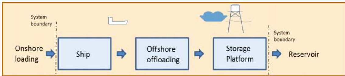
Figure 3-4: Third storage option: shipping to an offshore offloading point close to the injection site, with temporary storage and injection from the platform. Processing of the CO 2 takes place on the storage vessel or the platform.
