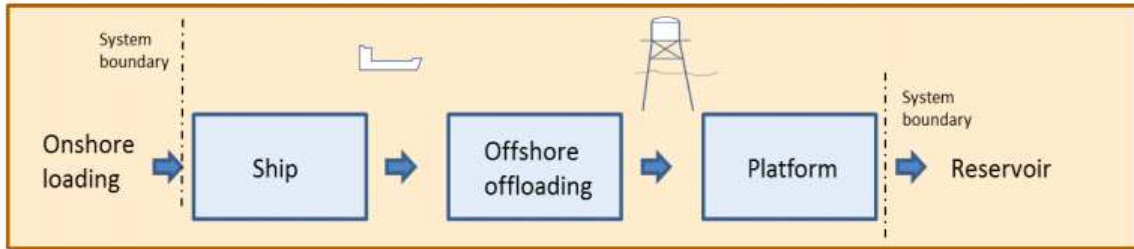
Figure 3-3: Second design option: CO 2 shipping to an offshore offloading point close to the injection site and injection from the platform. No intermediate offshore storage. CO 2 processing takes place both on the ship and platform.
